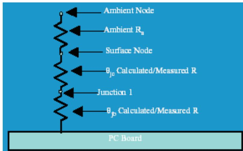
Figure 25. Thermal Resistance
