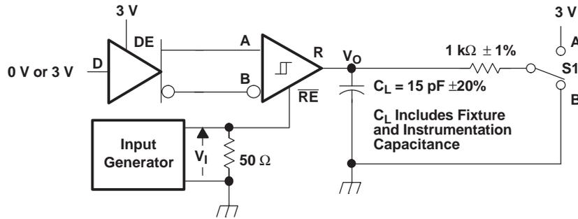
Generator: PRR = 500 kHz, 50% Duty Cycle,  $t_r < 6\text{ ns}$ ,  $t_f < 6\text{ ns}$ ,  $Z_o = 50\ \Omega$
